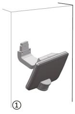
Fix the luminaire to the wall using the screw holes.
