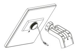
Attach the bracket marked "A" to the back of the solar panel (also marked "A") and tighten the hinge by hand.
