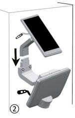
Slide the solar panel with bracket "B" onto bracket "A" on the luminaire and secure with
