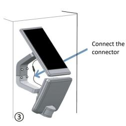
Connect the solar panel to the luminaire
